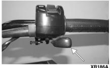
Control engine RPM with the position of the throttle lever. Operate this lever with the thumb. Pushing it forward increases engine RPM and allowing it to retract decreases engine RPM.
